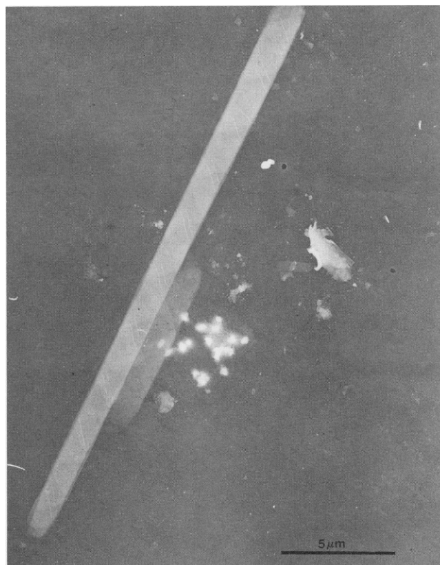
FIGURE 3 Transmission electron micrograph of unstained monomeric tubules. Such samples often show more wrinkling of the tubule walls than is apparent here. The smaller tubule appears to share a sheet of lipid with the larger, as the wrapping lines are continuous from one to the other. Scale bar, 5 \mu\text{m} .
